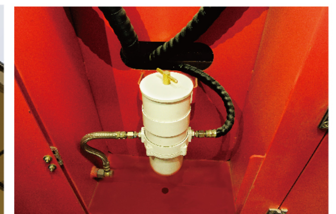
▪ Steel wire wined hoses are used and safety level is improved greatly.
