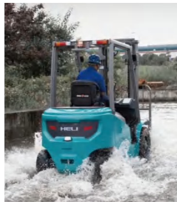
After 10mins wading test, the vehicle has no failure. (Water depth 200mm)
