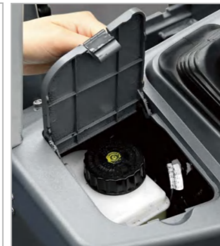
Brake fluid within reach, easy to check and refill
