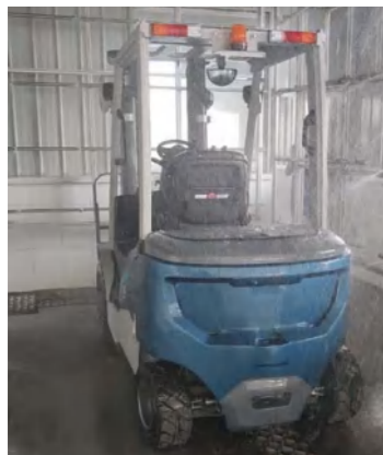
Rain Test: The whole vehicle is simulated to be under a short - duration rainstorm for 15 minutes (rainfall intensity is 5.43 mm/min) with live - load testing, and the vehicle can operate continuously without failure.
