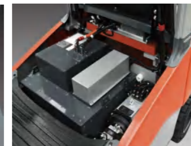
The electrical design is concentrated on the top of lithium battery, and the maintenance points are centralized, which is convenient for inspection and maintenance.
